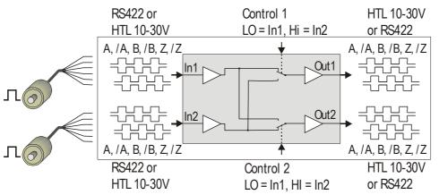
Both inputs can be individually set to either symmetric (differential) format using A, /A, B, /B, O, /O channels or to asymmetric (single-ended) format using A, B, O channels only.
