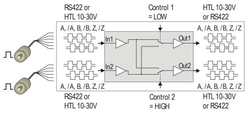
Both inputs can be individually set to either symmetric (differential) format using A, /A, B, /B, 0, /O channels or to asymmetric (single-ended) format using A, B, O channels only.
